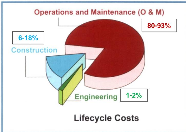
Figure 1: Typical breakdown of project life cycle costs
